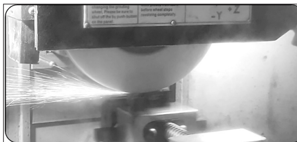
Fig. 3. Experimental setup used for carrying out grinding experiments and grinding wheel-workpiece interaction.
