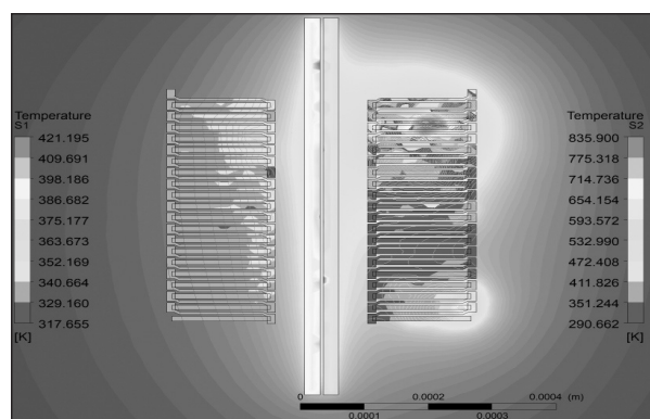
Fig. 10. Zoom-in view of the sensors inside the fluid flow, shows temperatures of sensor 1 & sensor 2 in direct flow model simulation.
