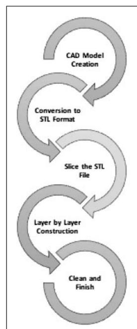
Fig. 1. Steps in 3D printing with FDM.
