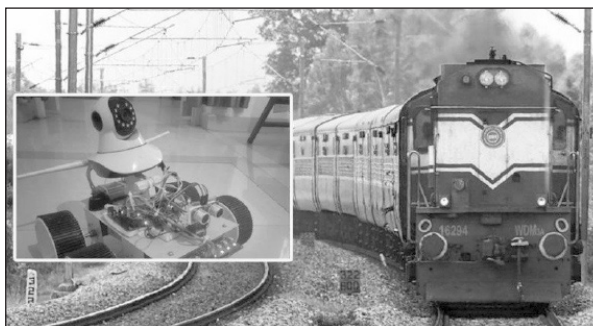
Fig. 8. A robot called USTAAD has been developed by the mechanical branch of the central railway's nagpur division, which analyses parts of the coach in real time with an HD camera and transmits them over Wi-Fi (Indian Railways, 2020).
