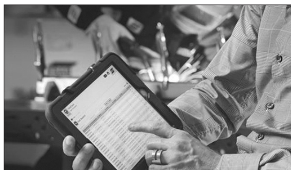
Fig. 6. Weld cloud online welding-data management system (Welding data collection, 2021).
