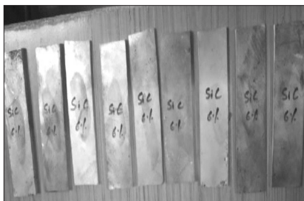
Fig. 8. Al 7178 - 6% SiC rolled samples.
