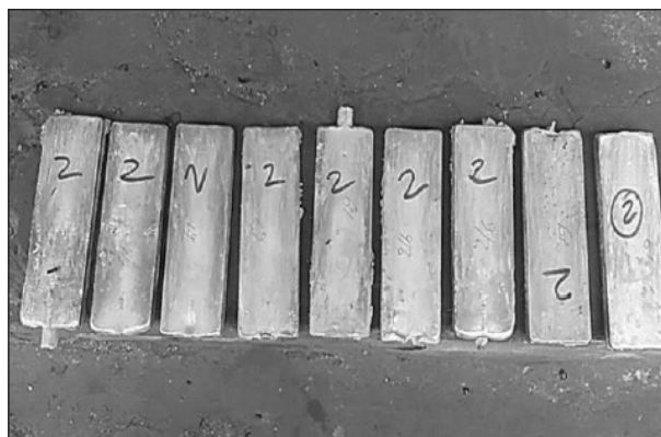
Fig. 4. Al 7178 - 6% SiC casting.
