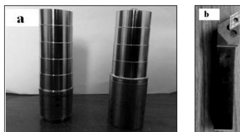
Fig 2 ( a & b). Photograph of Workpiece After Turning and Tool Used for the Machining
