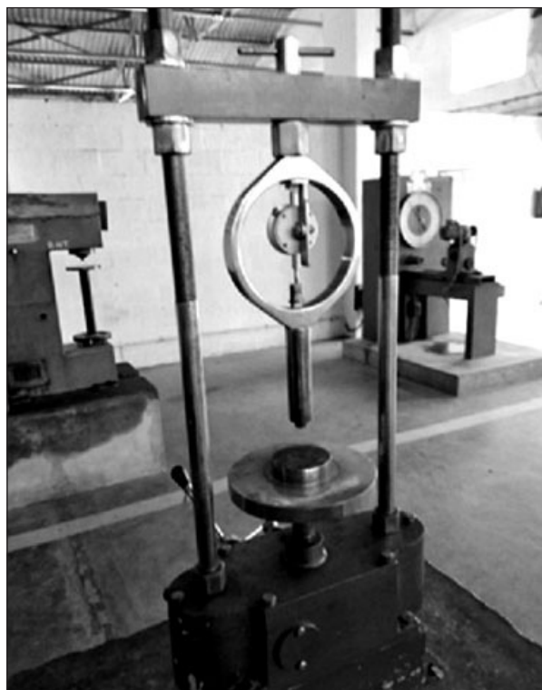
Fig 6. Brinell Hardness Tester
