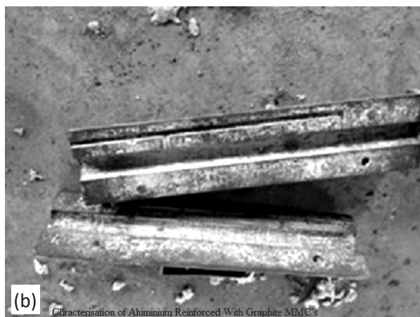
Fig 1. Die Used to Produce the Test Specimen
