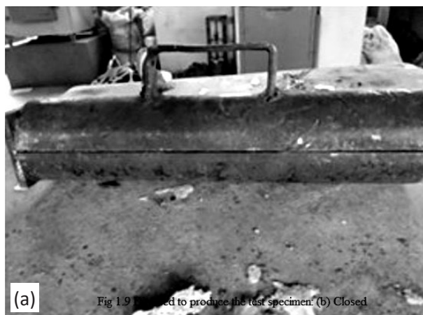
Fig 1. Die Used to Produce the Test Specimen
