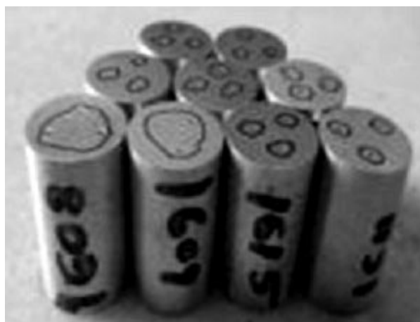
Fig 7. Hardness Test Specimen
