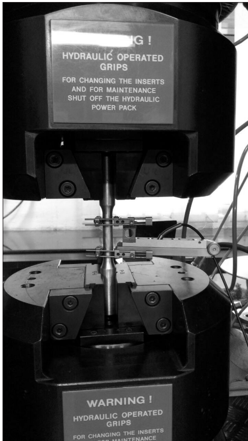
Fig 7. Attaching the Sensor to the Specimen
