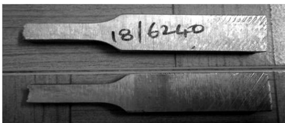
Fig: Tensile test Specimen after testing
