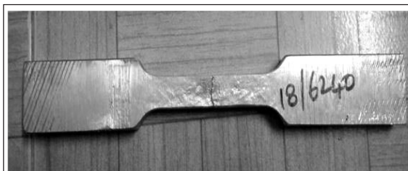
Fig: Tensile test Specimen before testing
