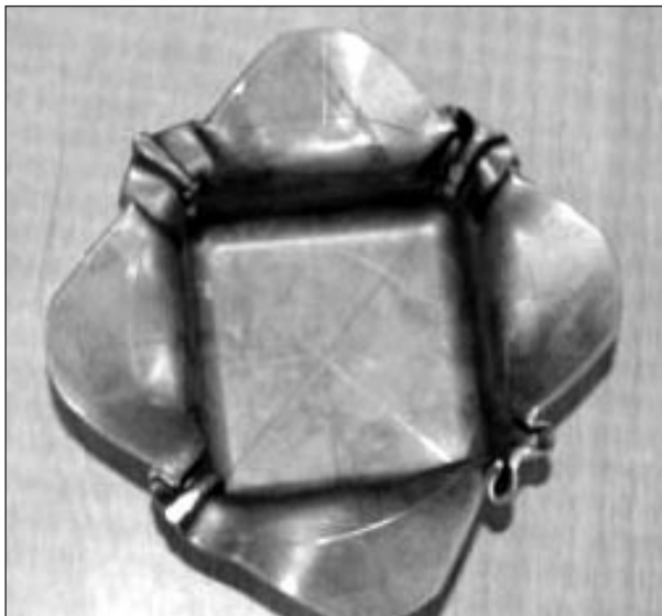
Fig 7. Square Bimetallic Cup with Cu Inside
