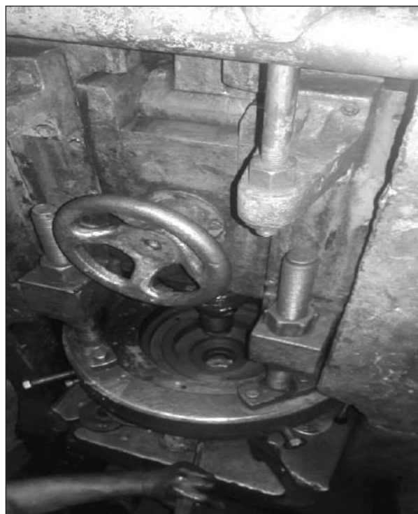
Fig 4. Hydraulic Press used to Draw Cups
