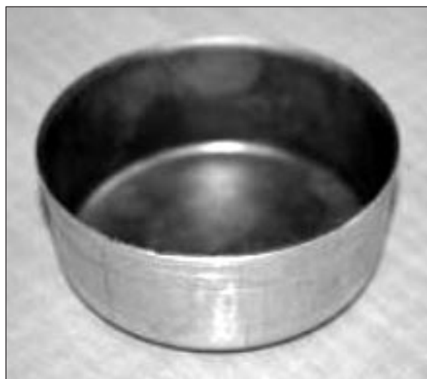
Fig 5. Cu- Ai Bimetallic Cup with Cu Inside
