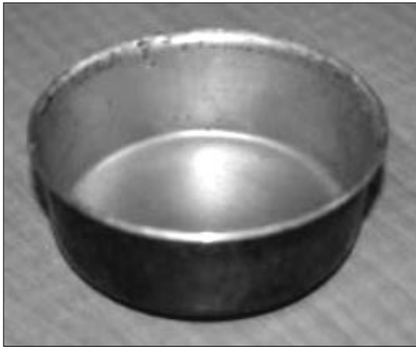
Fig 6. Cu- Al Bimetallic Cup with Al Inside
