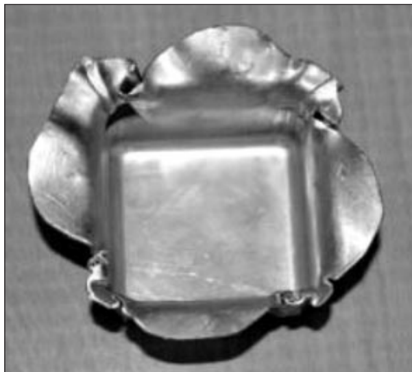
Fig 8. Square Bimetallic Cup with Al Inside
