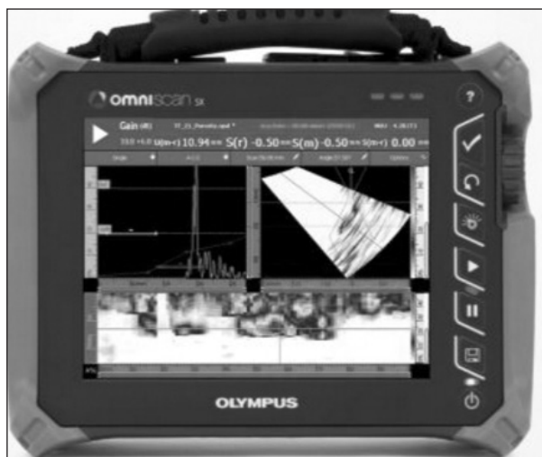
Fig 4. Phased Array Ultrasonic Testing Equipment with A, S and C Scan
