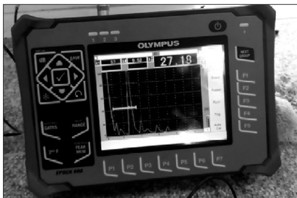
Fig 1. A- scan Presentation of Flaw Detection in Conventional UT
