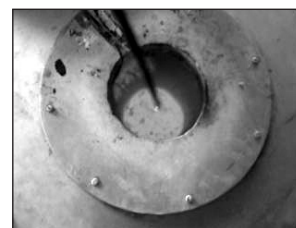
Fig 4.4. Molten Metal in furnace
