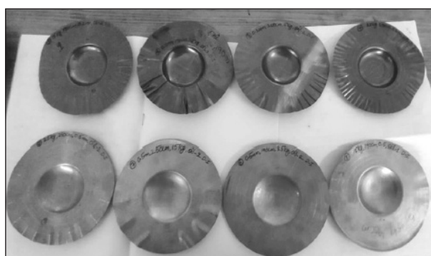
Fig. 2. Deformed superni 718 work pieces.
