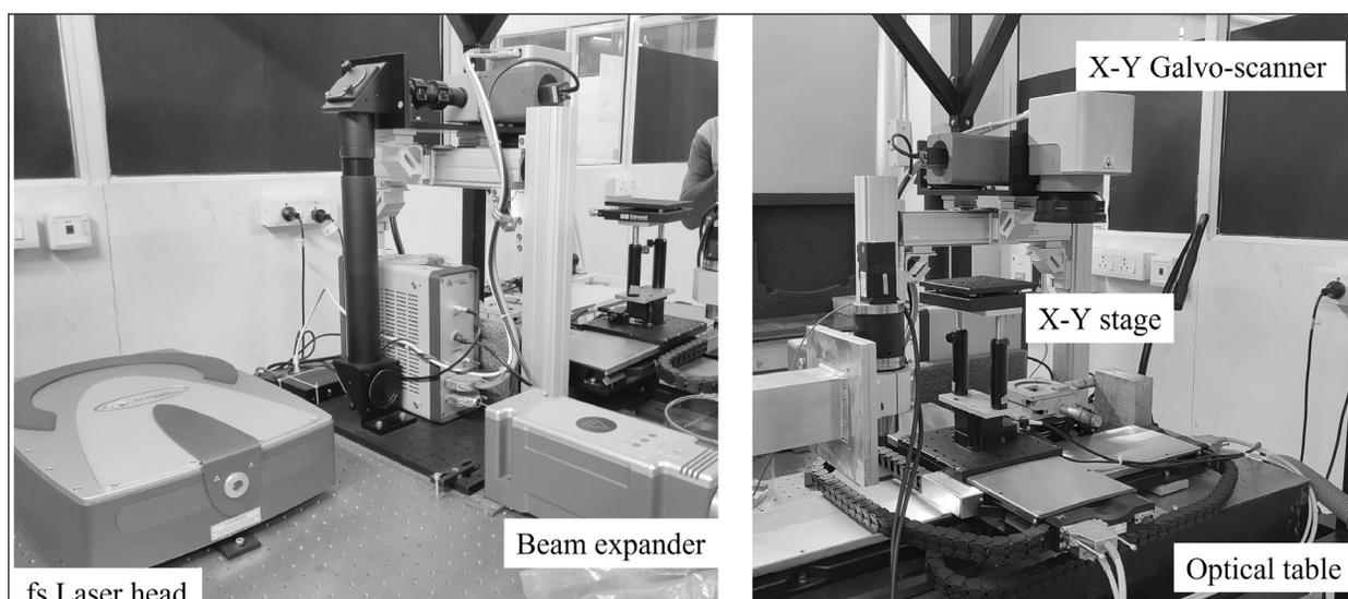
Fig. 1. Experimental setup of the ultrafast femtosecond laser.
