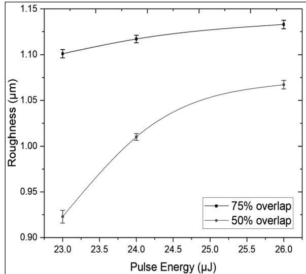
**Fig. 4.** Effect of pulse energy on surface roughness.
