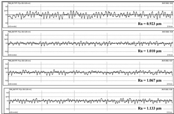
**Fig. 3.** Surface roughness profiles of the micro-milled region of the PC sheet.
