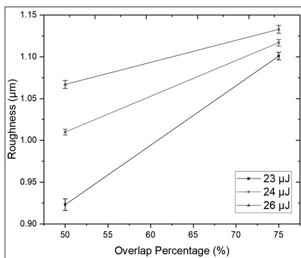
Fig. 5. Effect of pulse overlap percentage on surface roughness.
