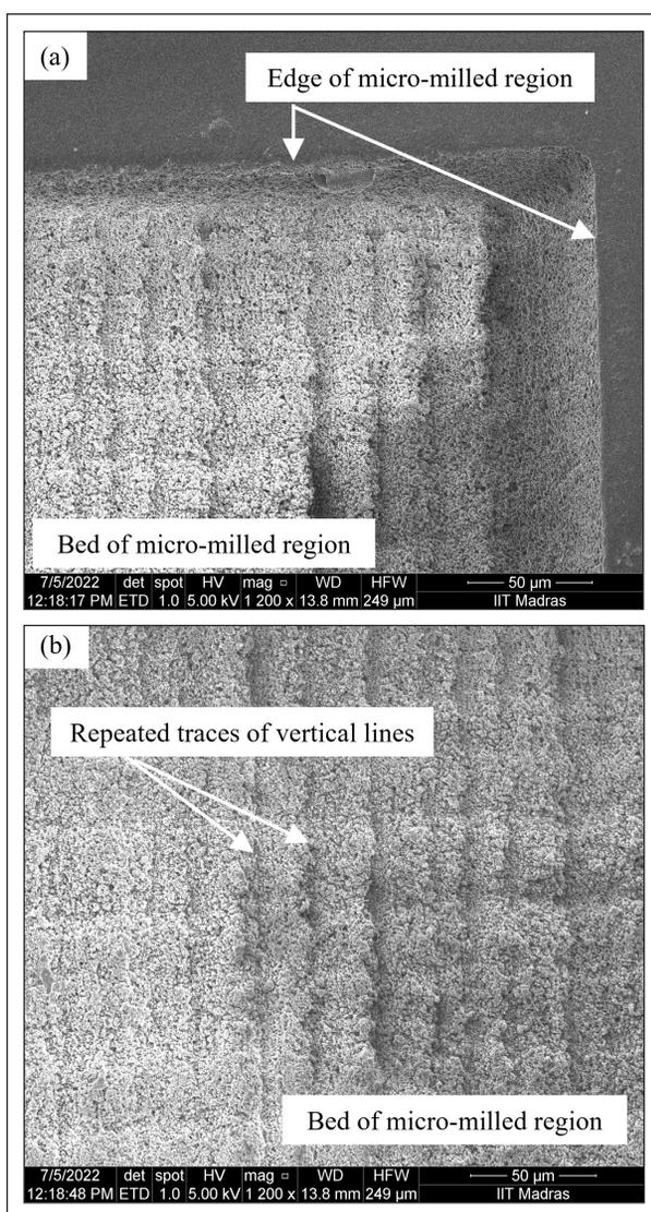
Fig. 2. FESEM images on (a) the edge and (b) the bed of the micro-milled region of the PC sheet.
