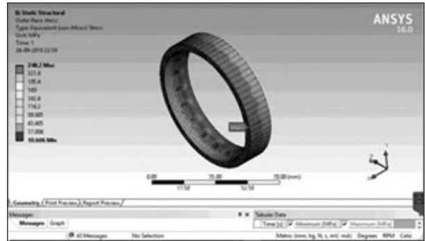
Fig 11. Von Mises Stress in Outer Race
