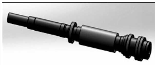
Fig 2. SOLIDWORKS Drawing of the Spindle with Bearings
