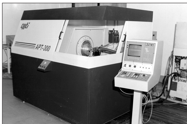
Fig 2. The Diamond Turning Machine Used for Experimental Work
