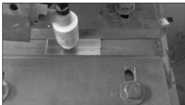
Fig. 3. Clamping of joint for welding.
