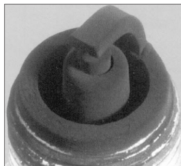
Fig. 3. Carbon deposited electric spark plug.
