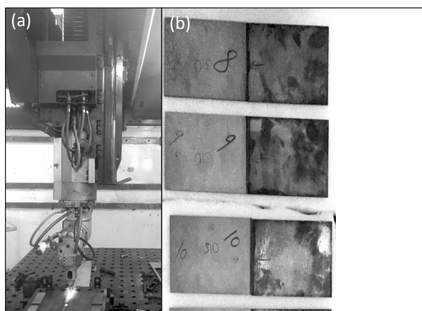
Fig. 1. (a). LBW experimental process and (b). welded work pieces.
