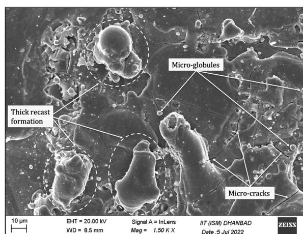
Fig. 4. Machined region on Ti-grade 5 workpiece.
