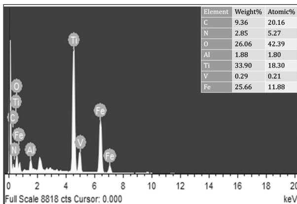
Fig. 5. EDS report of machined workpiece surface.
