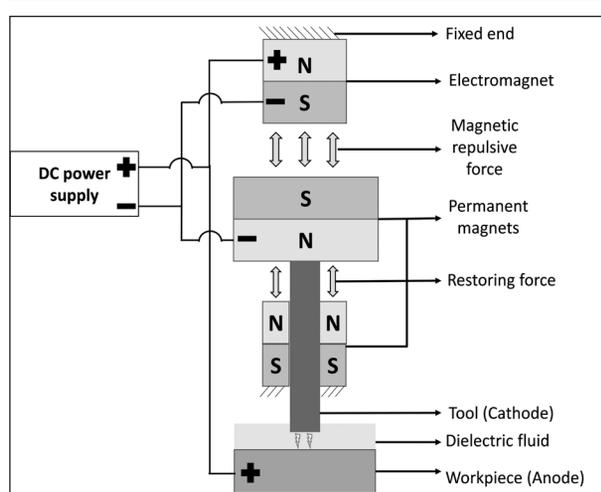
Fig. 1. Schematic illustration of Maglev EDM mechanism.
