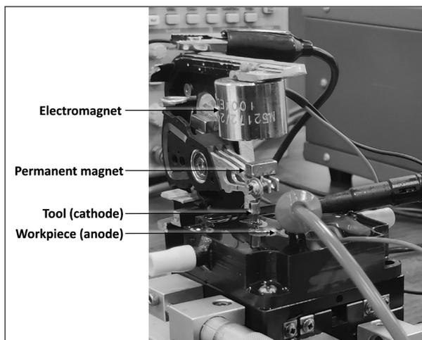
**Fig. 2.** Maglev EDM setup and its components.
