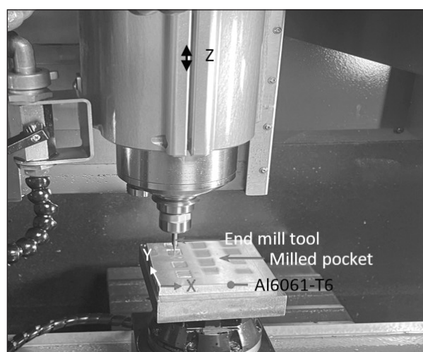
Fig. 2. Conventional milling setup for generating pockets.
