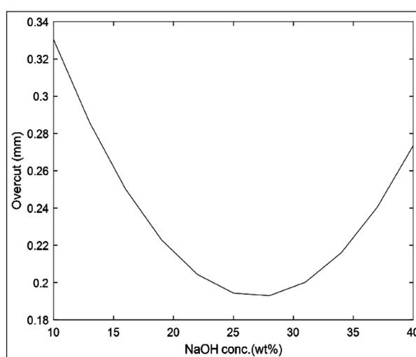
Fig. 5. Effect of NaOH conc. on overcut.
