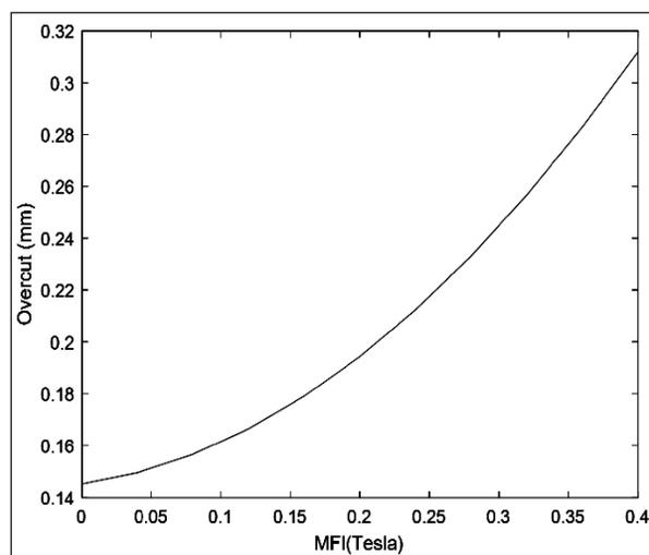
Fig. 7. Effect of magnetic field on overcut.
