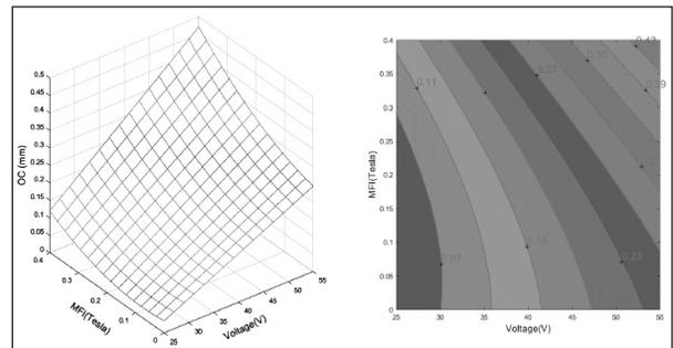
Fig. 10. Effect of voltage-MFI on overcut (NaOH conc.-25 wt%, TRS-90 rpm).
