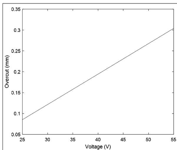
Fig. 4. Effect of voltage on overcut.
