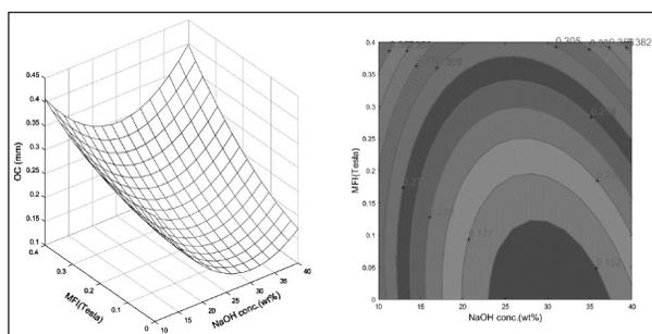
**Fig. 12.** Effect of NaOH conc.-MFI on overcut (voltage-40 V, TRS-90 rpm).
