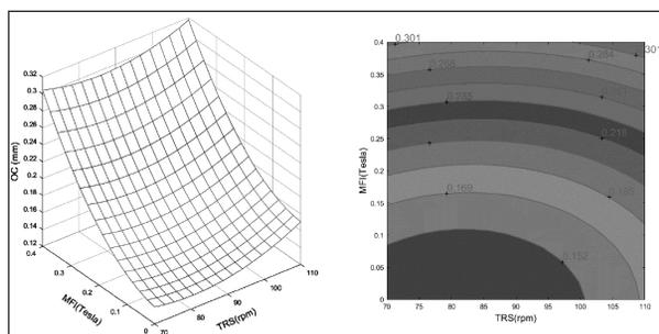
**Fig. 13.** Effect of TRS-MFI on overcut (voltage- 40 V, NaOH conc.- 25 wt%).
