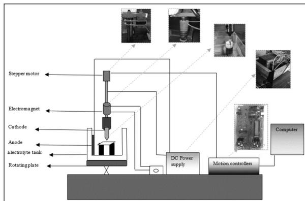
Fig. 1. Schematic diagram of MF-ECSD setup (Singh et al., 2022a; Singh et al., 2022b).
