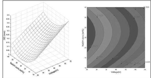
Fig. 8. Effect of voltage-NaOH conc. on overcut (TRS- 90 rpm, MFI-0.2 T).
