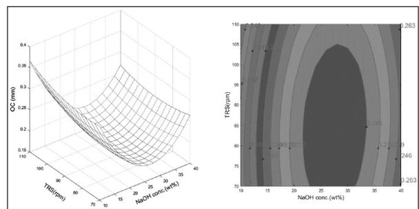
Fig. 11. Effect of NaOH conc.-TRS on overcut (voltage-40 V, MFI-0.2 T).
