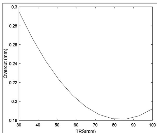
Fig. 6. Effect of tool rotational speed on overcut.
