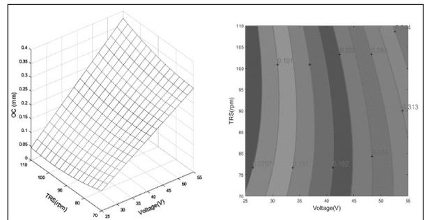
Fig. 9. Effect of voltage-TRS on overcut (NaOH conc.-25 wt%, MFI-0.2 T).
