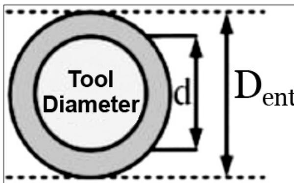
Fig. 3. Schematic diagram for computing overcut (Rajput et al., 2020).
