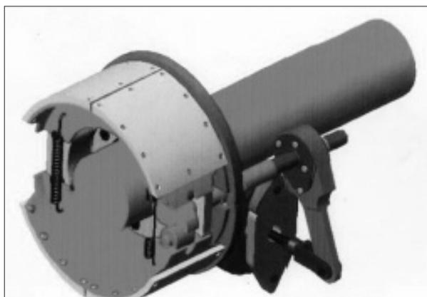
Fig. 5. Brake drum assembly
