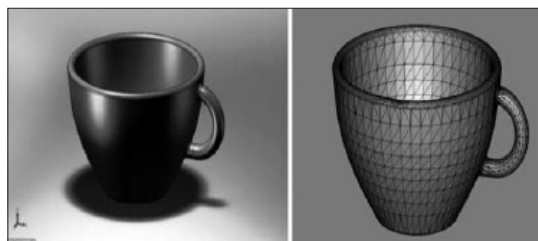
Fig 4.1a. CAD model onto left is converted into STL (Standard triangulation language) format on the right.
