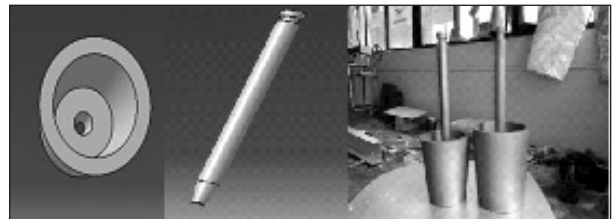
Fig. 10. Bottom pouring graphite crucible with tapping rod.
