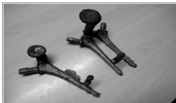
Fig. 13. As cast part: fabricated using RP
