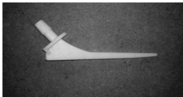
Fig. 5. RP Pattern fabricated on 3D printing machine.
