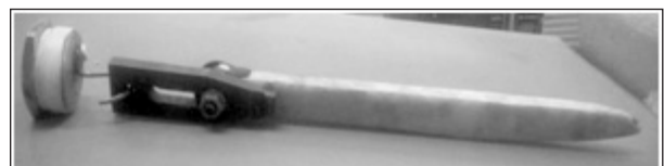
Fig. 11. Bottom pouring graphite crucible with tapping rod.
