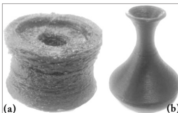
Fig. 5. (a) Quality of print when bearing had clearance; (b) Print quality after installing injection moulded bearings
