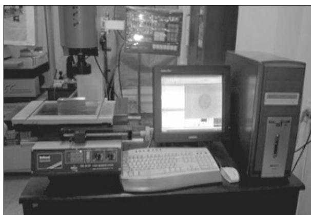
Fig. 3.10. Measurement of a sample hole diameter.
