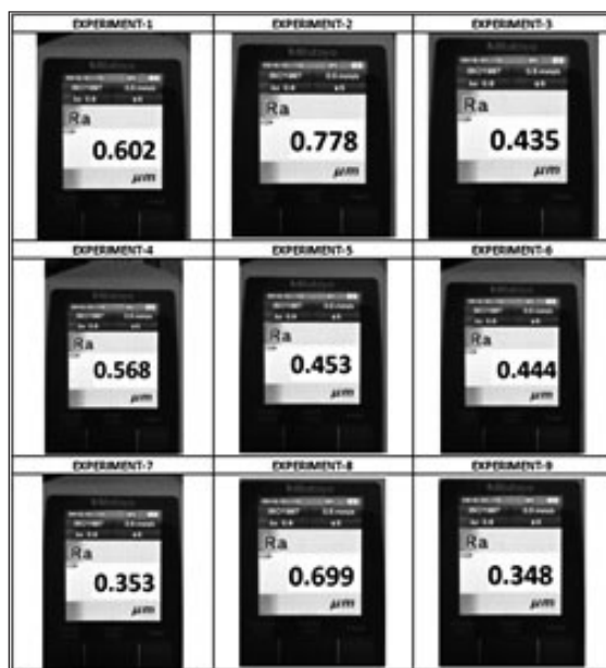
Fig.5. Experimentation on surface roughness.
