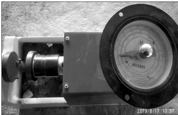
Fig. 1. Compression Strength testing device
