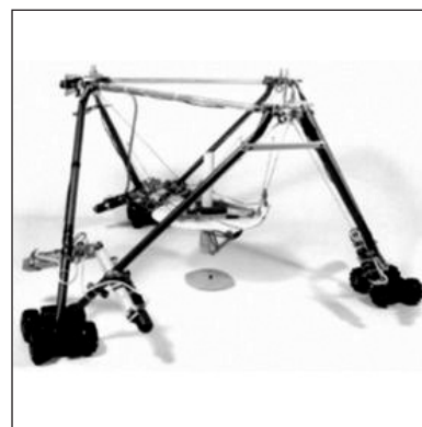
Fig. 5. Cable driven robot (Tang, 2014).
