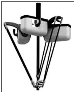
Fig. 4. Delta robot (Patel & George, 2012).
