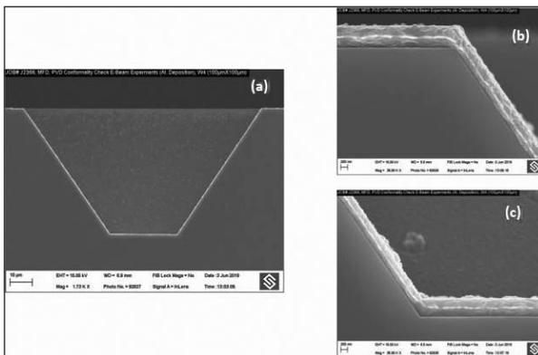
**Fig. 7.** Scanning electron microscopy images for cavity dimension of 100 x 100, (b & c) Cross-sectional image of Al metal at rotation speed of 25% of max rpm.
