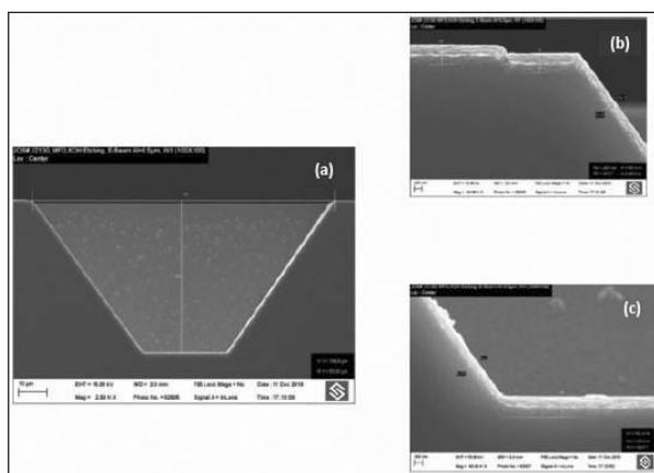
**Fig. 4.** (a) Scanning electron microscope images for wet etched cavity of dimension 100 x 100, (b & c) Cross-sectional image of Al metal deposited at Top and Bottom edge of cavity at set rotation speed of 12 % of max rpm.
