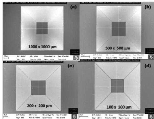
Fig. 3. Scanning electron microscopy images of KOH etched trenches in silicon wafer.
