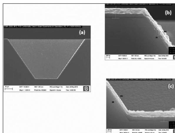
**Fig. 5.** (a) Scanning electron microscopy images for wet etched cavity of dimension 100 x 100, (b & c) Cross-sectional image of Al metal deposited at top and bottom edge of cavity at rotation speed of 25 % of max rpm.
