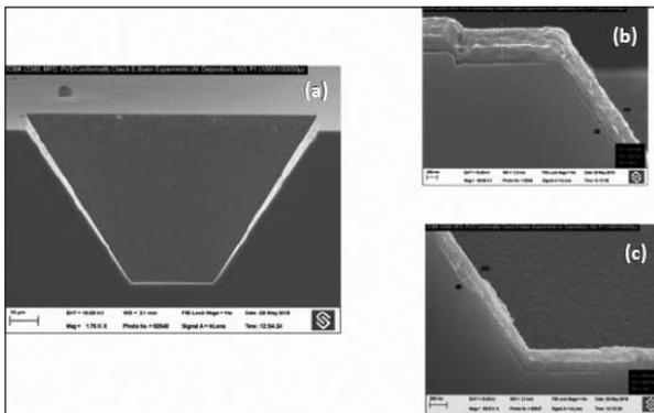
**Fig. 6.** Scanning electron microscopy images for cavity dimension of 100 x 100, (b & c) Cross-sectional image of Al metal at rotation speed of 12 % of max rpm.
