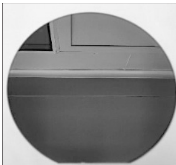
Fig. 2. Thin-film metal deposited 6-inch silicon wafer.
