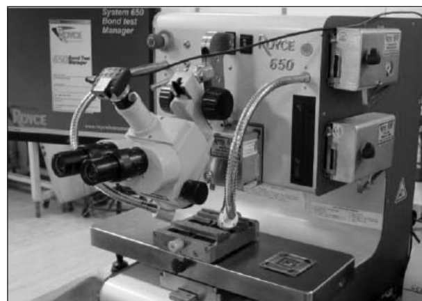
Fig. 10. Bond strength test equipment.
