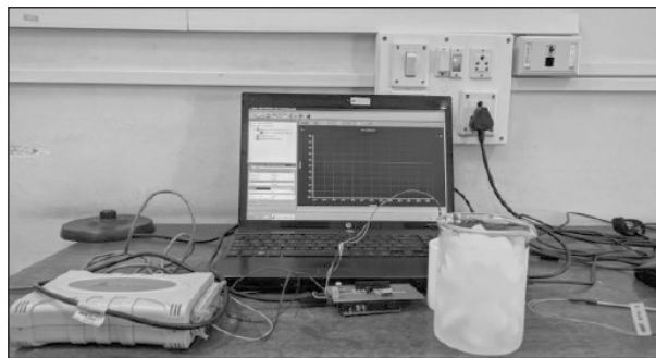
Fig. 17. Ice bath test setup for response time measurement.
