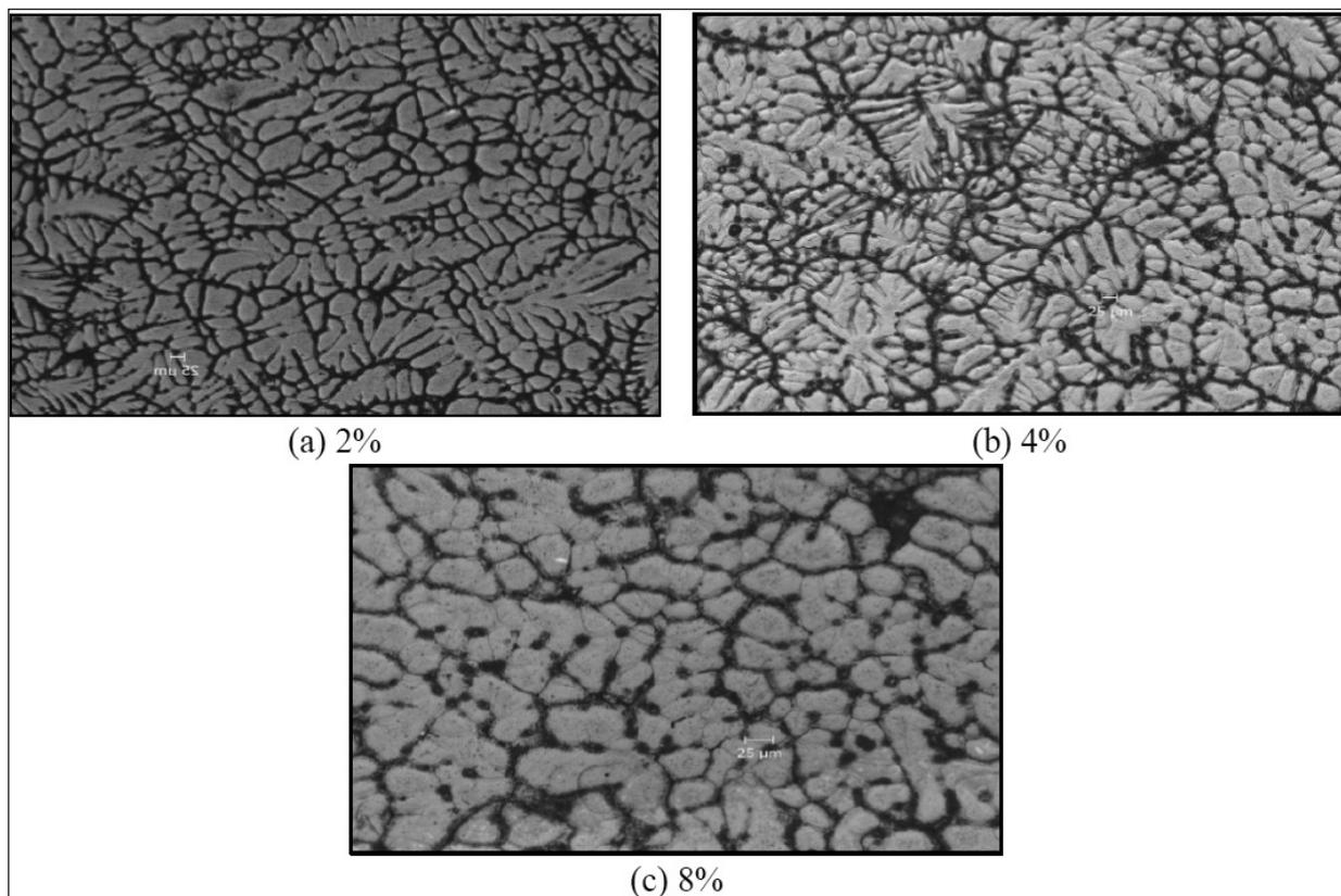
Fig. 2. Optical microstructure of AA6061/SiC composites.
