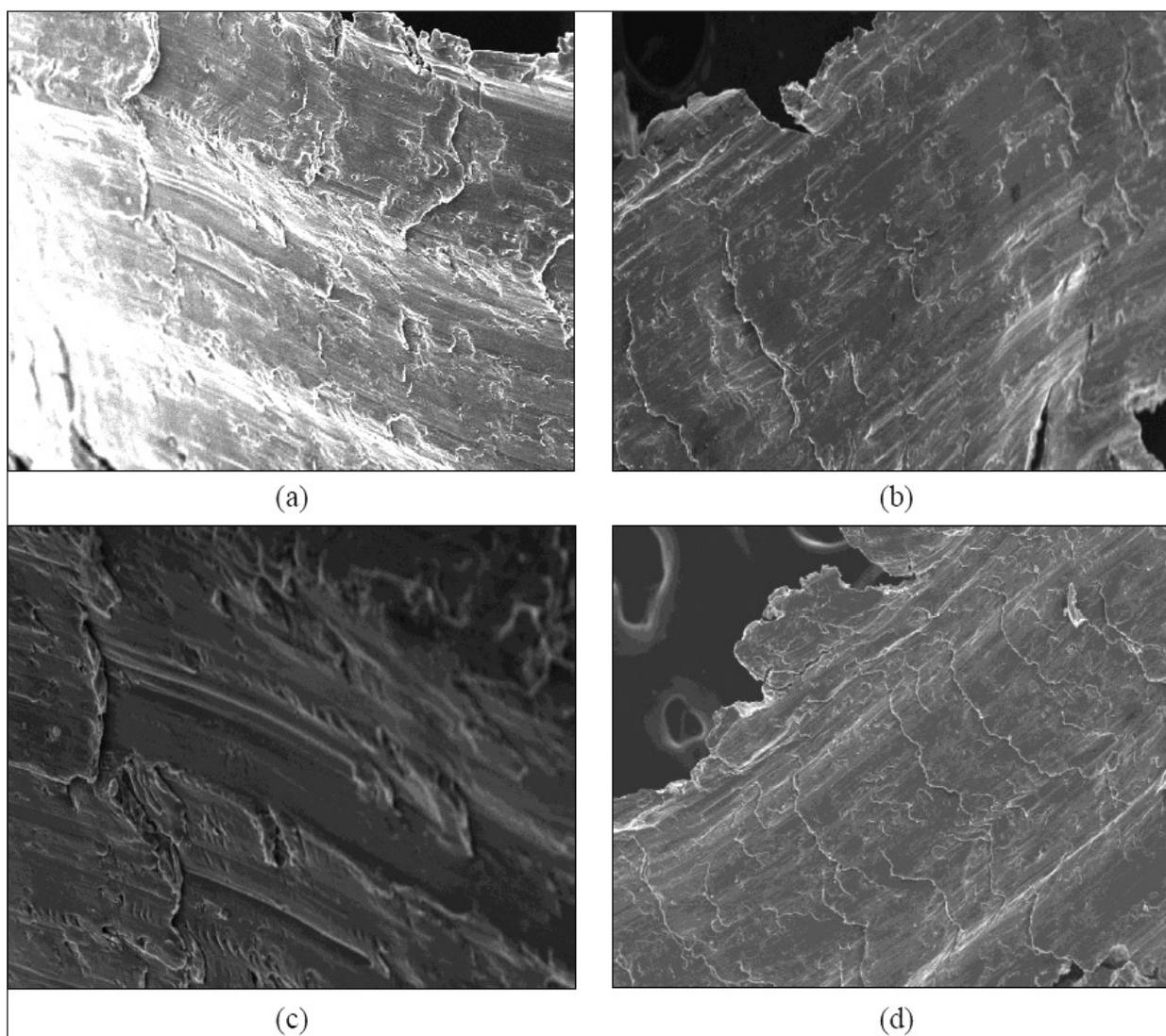
**Fig. 5.** Chip morphology for (a) 2%, (b) 4%, (c) 6% and (d) 8% SiC reinforced AA6061 composites at depth of cut of 0.3 mm, speed 180 rpm and 0.6 mm/rev.
