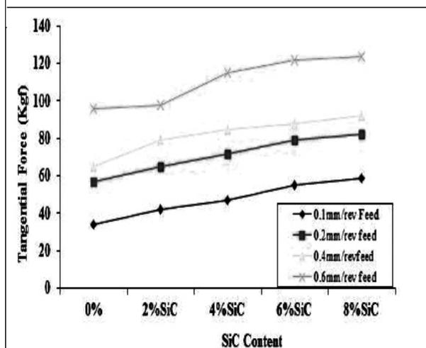
(c) Depth of cut – 0.6 mm, Speed – 180 rpm
