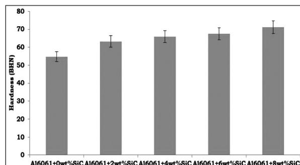
Fig. 3. Brinell hardness of AA6061/SiC composite.
