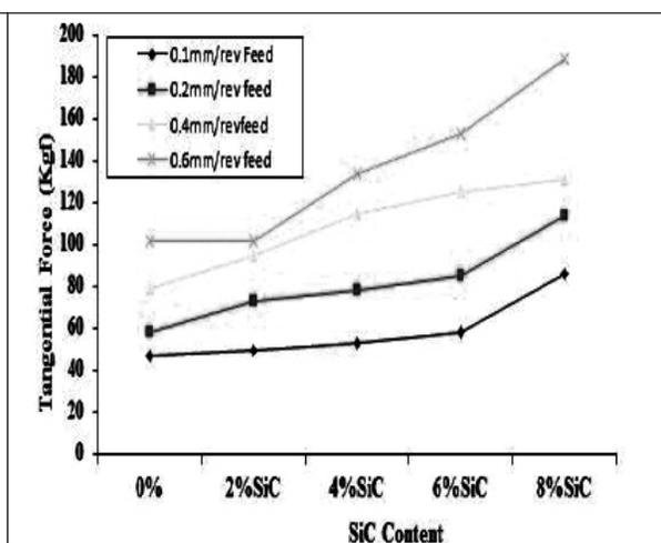
(b) Depth of cut – 0.3 mm, Speed – 280 rpm
