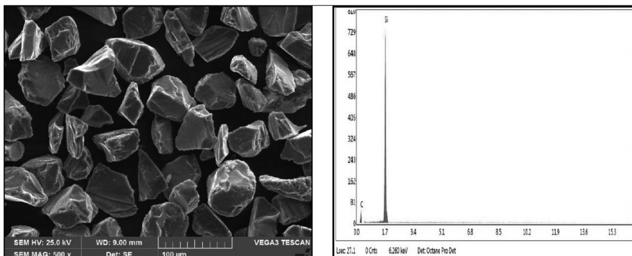
Fig. 1. (a) SEM image and (b) EDS of SiC particles.
