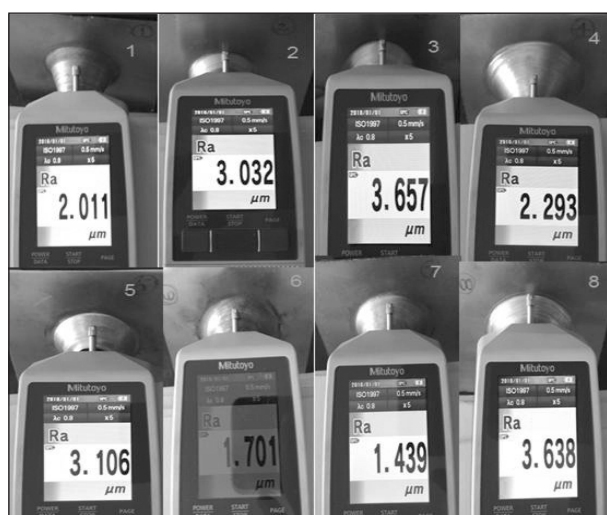
Fig. 4. Experimentation on surface roughness.
